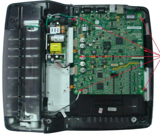
6. Remove the M3x4 CSK screws securing the patient cable connector to the PWA.
