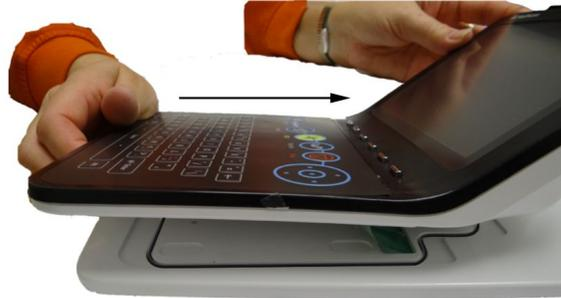
9. Turn over the top cover assembly and use a cross-head screwdriver to secure the display assembly to the top cover with the six screws.
