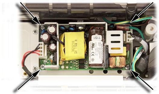
6. Lift the power supply assembly from its base.
