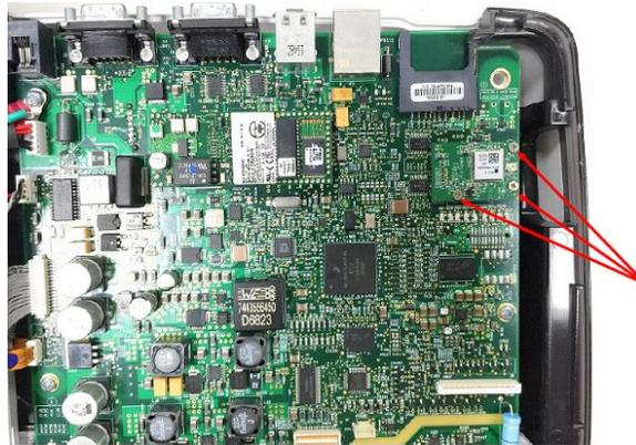
4. Gently detach the embedded wireless module from the main board.
