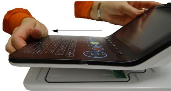
5. Turn the display over so the bottom display cover is facing you.
