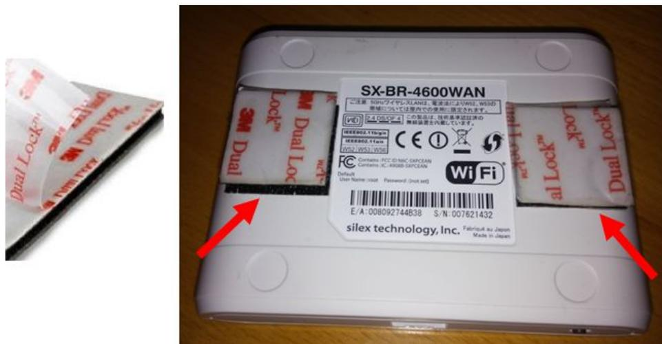
3. Peel the adhesive liner from the Dual Lock stuck on the Silex module (on either side of the label) as shown in step 2. Carefully position the Silex Module on the
