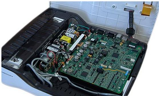
The top cover assembly, with the display assembly mounted on it, is now completely separated from the device.
