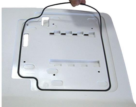
7. Align the tabs on the display bottom cover with the slots on the device top cover.
