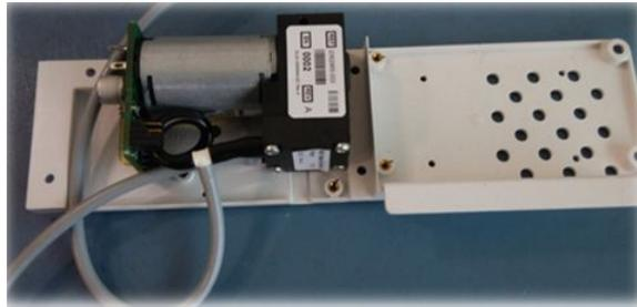
The following instructions describe how to remove the defective KISS pump assembly and install the new KISS pump assembly.
