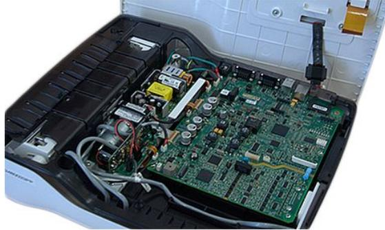
2. Gently lower the top cover assembly part way and connect the display cable (1) and keypad ribbon (2) to the PWA.
