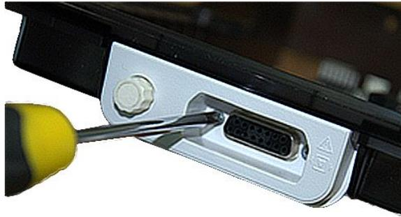
5. Using a cross-head screwdriver, remove the patient cable connector from the main board.
