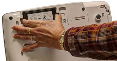
6. Place the new battery in the compartment and push until it clicks into place.
