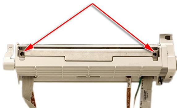
4. Reattach the printer module assembly to the bottom cover.
