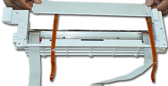
2. Holding each end of the printer module assembly, gently push out the end pieces and use your thumbs to slide the crossbar into position.
