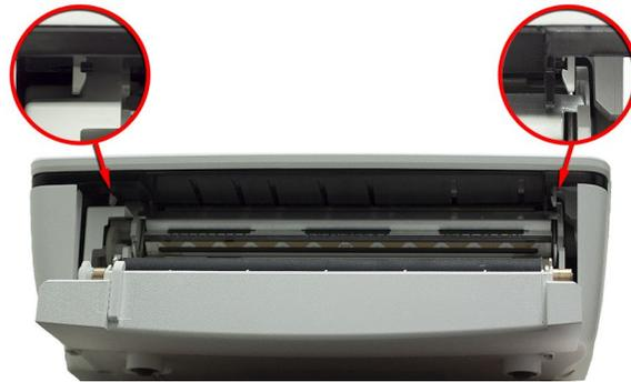
4. Using a flat-head screwdriver, gently disengage the top cover from the latches.
