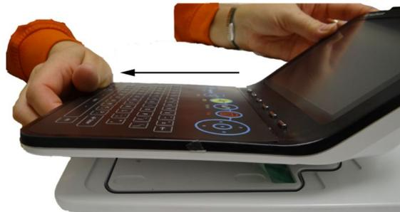
3. Turn the display over so the bottom display cover is facing you.
