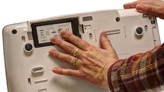
2. Replace the cover on the battery compartment.
