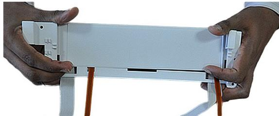
3. Snap the two end pieces back into place and secure them to the printer module assembly with two fasteners on each end.
