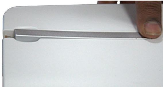
6. Grasp both sides of the raised printer door release lever, and lift to remove it from the top cover.
