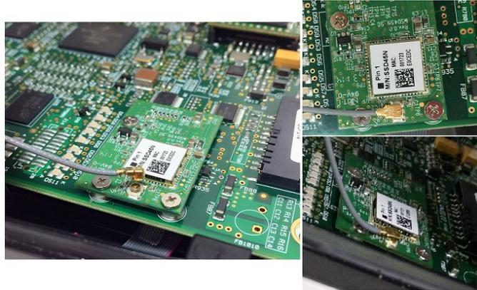
4. Thread the antenna through the clips.
