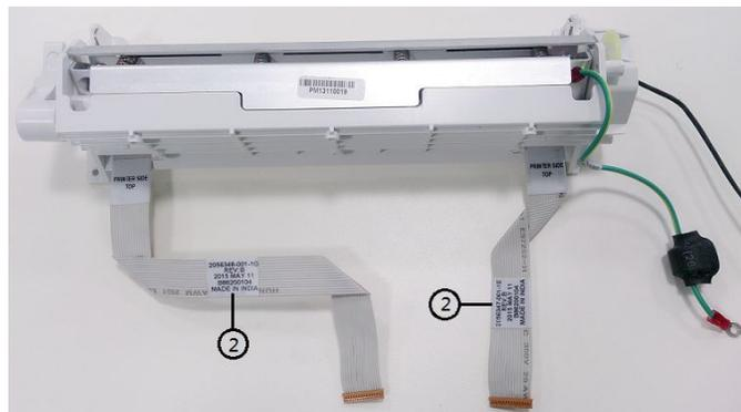
Make sure the connectors are latched properly to avoid any partial contacts.
