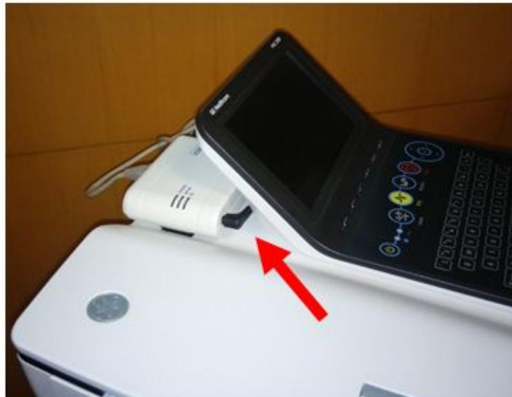
4. Route and connect the Ethernet and USB Power cables from Silex module to the MAC2000 unit.
