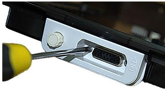
3. Secure the PWA to the chassis by inserting and tightening the screws.
