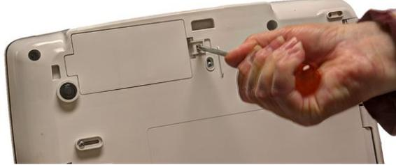
2. Push the tab to remove the battery compartment cover.
