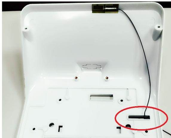
4. Replace the display bottom cover, carefully threading the keypad ribbon and display cable through the openings.
