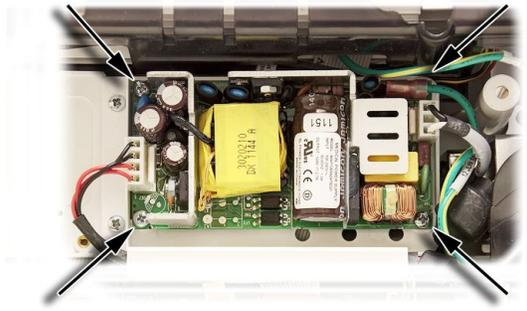
3. Attach the power supply harness to the PWA.
