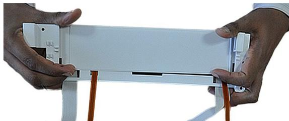
6. After it clears the end pieces, remove the crossbar with the two paper sensors.
