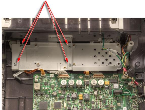
6. Lift the power supply/KISS pump base from the chassis.
