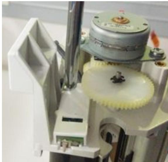
3. Route the sensor cable through the groove provided on the door sensor cover. Care should be taken to avoid cable pinch. Fasten the assembly using M3 x 8 screw provided in the kit with a torque of 4.7 Kgfc<sub>m</sub>.
