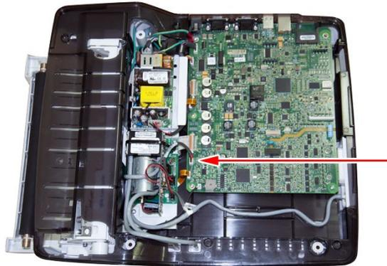
4. Attach the KISS pump tubing to the locations identified in the following photograph.
