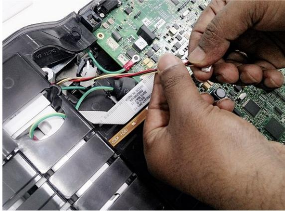
7. Connect the cables and harnesses to the PWA.
