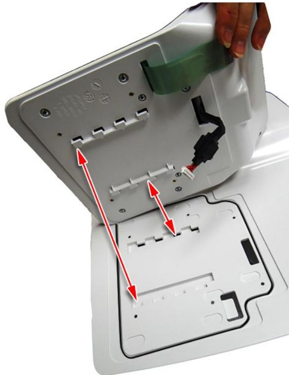
6. Lower the display bottom cover toward the device top cover and carefully thread the display cable and keypad ribbon through the slots on the top cover.
