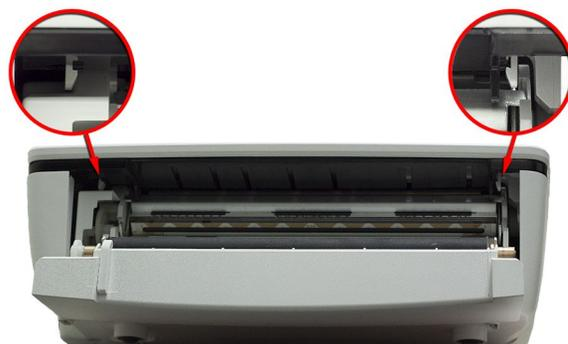
6. Using a flat-head screwdriver, gently disengage the top cover from the latches.
