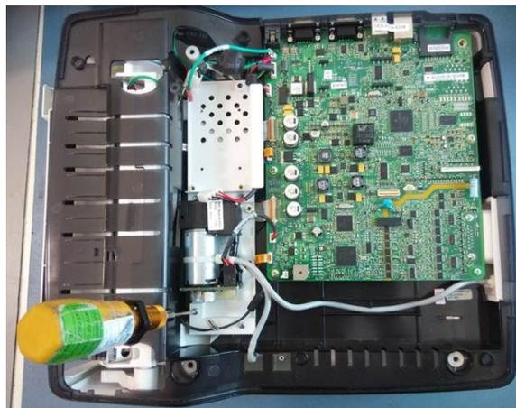
4. Re-assemble the Power Supply to the KISS Pump plastic base using M3X5 (qty: 2) and M3X8 (qty: 2) screws.
