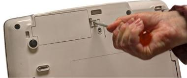
3. Push the tab to remove the cover of the battery compartment.
