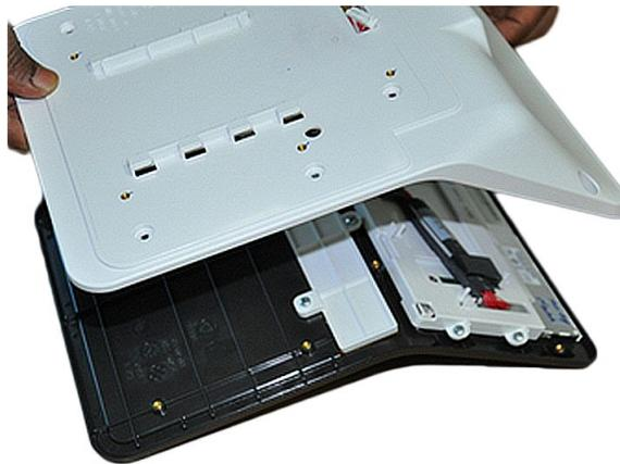
The bottom cover is now removed from the display assembly.
