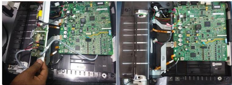
2. Pick the FRU-KISS pump assembly with base (PN: 2066261-069)" from the FRU shipping box and attach it to the color chassis by re-using existing fasteners M3X5 (qty: 4).
