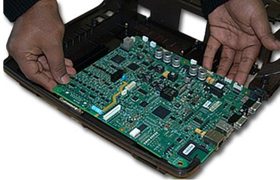
2. Connect the patient cable connector to the main board and use a cross-head screwdriver to secure it with two M3x4 CSK screws.
