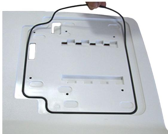
5. Align the tabs on the display bottom cover with the slots on the device top cover.
