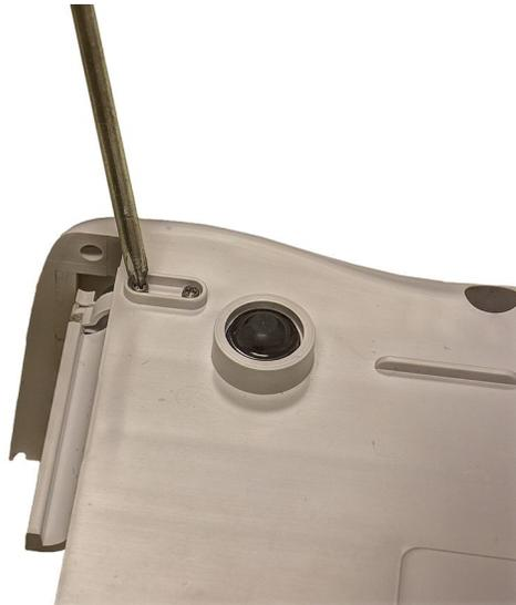
7. Turn the bottom cover over and remove the dampers on the either side of the printer door.
