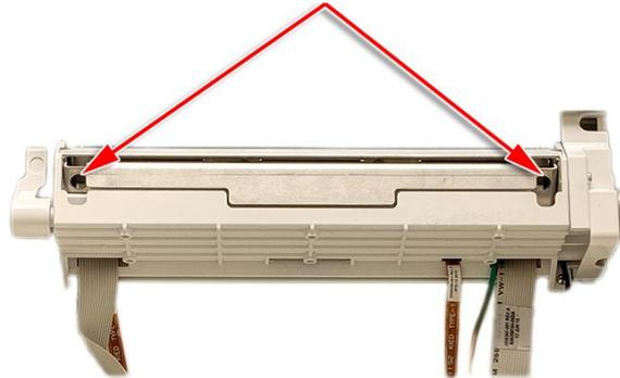
4. To remove the print head, gently lift it from the metallic print head holder, and carefully thread the two printer ribbon cables through the printer module assembly casing.
