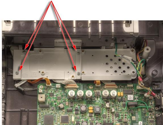
5. Lift the power supply/KISS pump base from the chassis.
