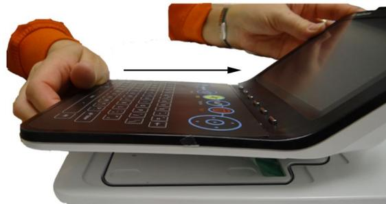
10. Turn over the top cover assembly and secure the display assembly to the top cover using the six fasteners.
