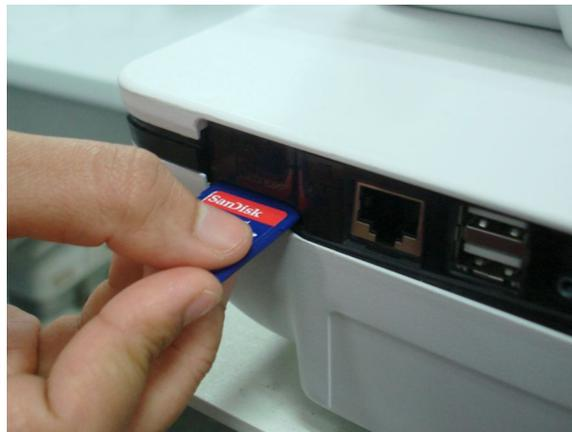
2. Push the SD card into the slot to seat it in place.
