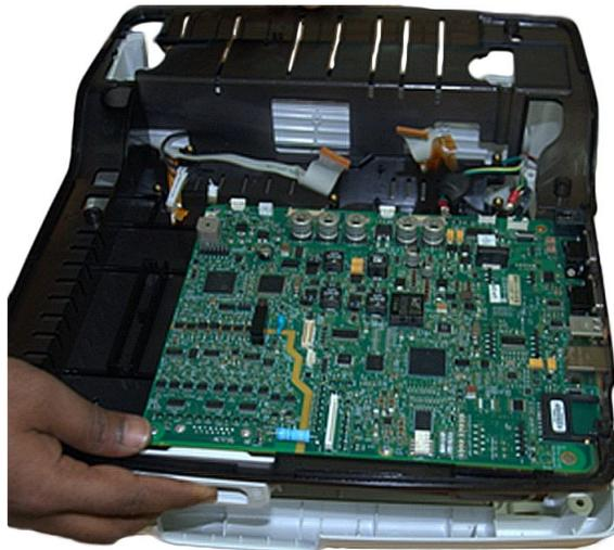
You have now detached the chassis and PWA from the bottom cover. You can now service the printer assembly or continue to remove the bottom cover. To service the printer assembly, see ["Printer" on page 139](#) . To remove the bottom cover, see ["Bottom Cover" on page 132](#).
