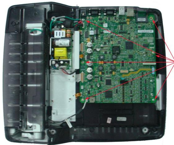
4. Using a cross-head screwdriver, remove the two M3x4 CSK screws securing the patient cable connector to the main board.
