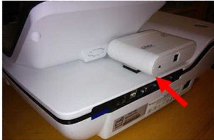
Ensure that, there is no pinching of the USB Power cable by the Display housing while routing the cable.
