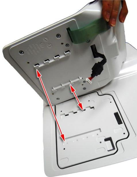
8. Lower the display bottom cover to the device top cover and carefully thread the display cable and keypad ribbon through the slots on the top cover.
