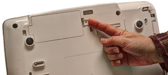
4. Using a cross-head screwdriver, tighten the screw securing the battery cover.
